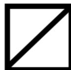
Structure is significantly damaged. Some areas are relatively safe, but other areas may need shoring, bracing, or removal of falling and collapse hazards.
