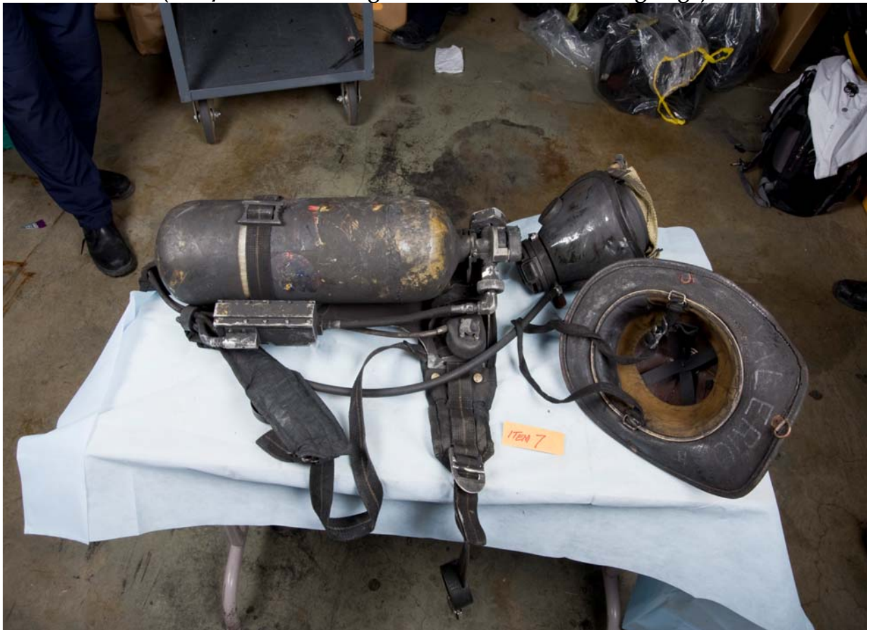
Victim 1's SCBA low pressure hose. This hose was cut during rescue operation (hose/mask was wedged under vehicle's tire in garage).
