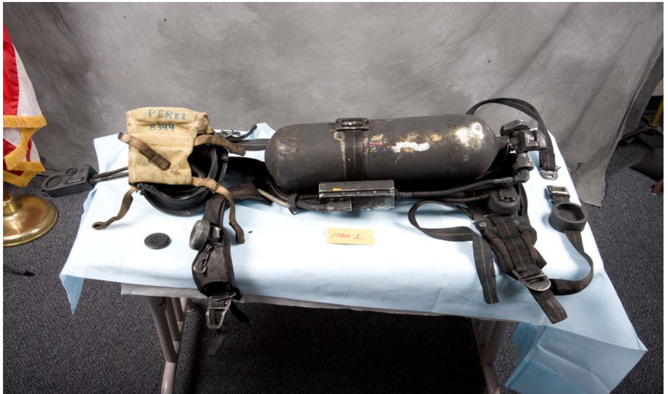
Victim 1's SCBA note the heavy sooting
