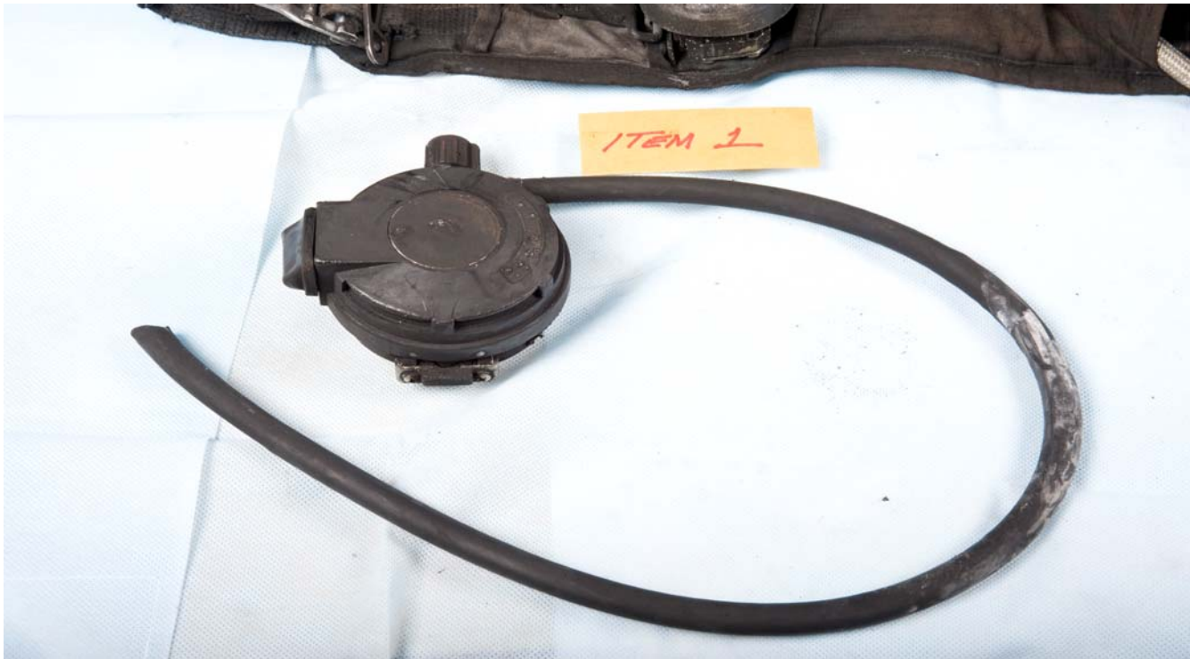
Victim 1's SCBA low pressure hose. This hose was cut during rescue operation (hose/mask was wedged under vehicle's tire in garage).
