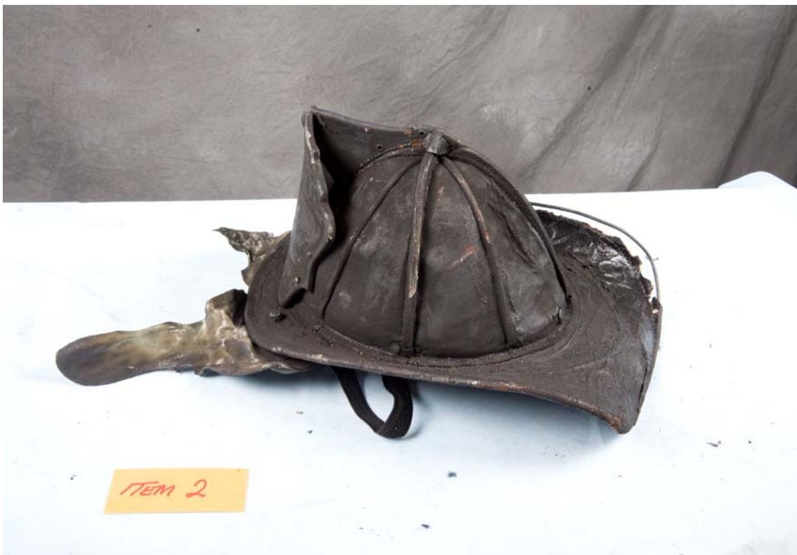
Note heat damage to helmet and the carbon material on the helmet
