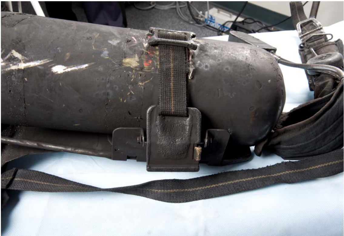
Note amount of carbon material that has been baked onto the SCBA of Victim 1
