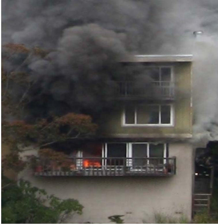
Color of the smoke being generated, indicates a hot and high carbon based fire
