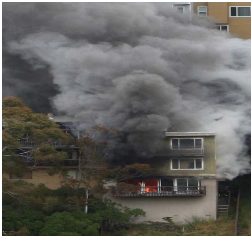
10:59:58 Note second window from the left has failed. Smoke conditions continue to change, due to application of water. (6582)
