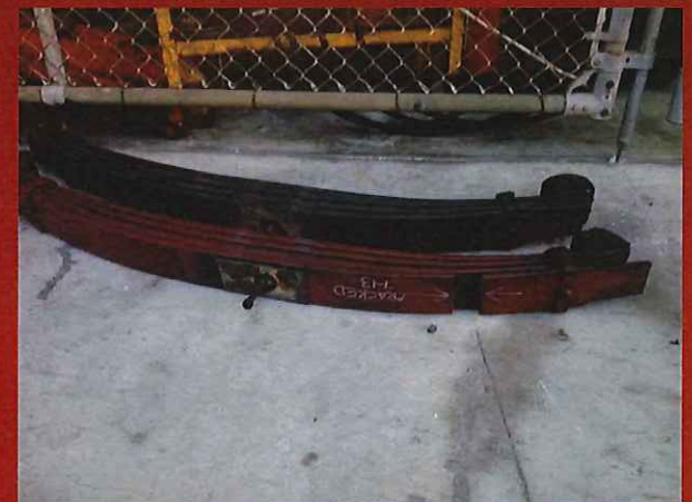
Cracked Leaf Springs
