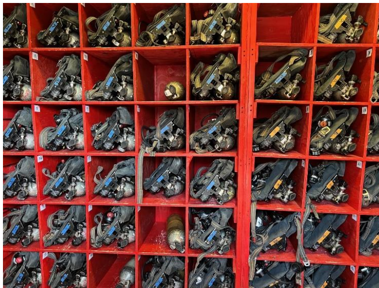
Inventory of SCBA packs, and reinforce shelving
