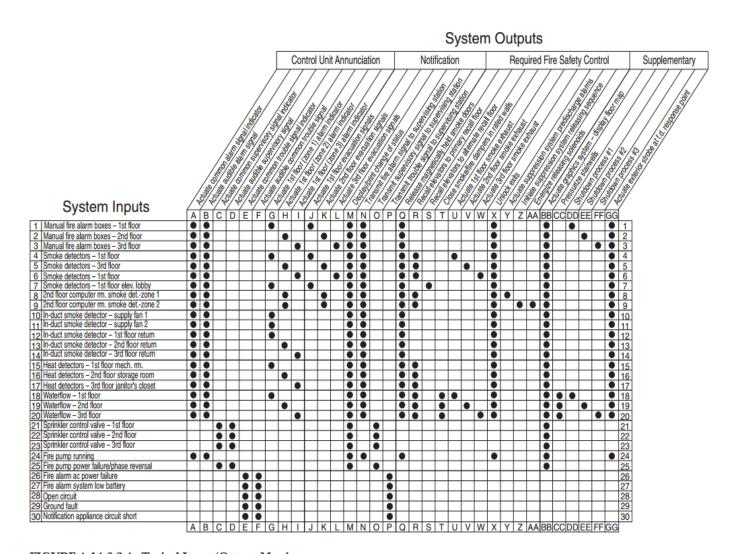
FIGURE A.14.6.2.4 Typical Input/Output Matrix.
